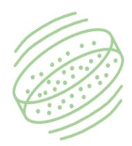
The newly developed Sand Resistance Test, or SRT, measures scratch resistance using sand as the medium. It consists of 300 shake-cycles in a sand tray and is supervised by a third-party technician.
