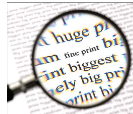
FIG. 2 Trivex material has a very high Abbe value of 45. The higher the Abbe value, the less the chromatic aberration as illustrated here.
