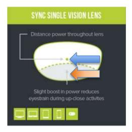
Fig. 2 Comparison of a single power (focus) single vision lens vs. Sync III with slight power boost
